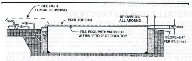
FIG. 1 - PREPARATION FOR CONCRETE OR PAVER BLOCK DECK INSTALLATION
