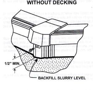
NOTE: KEEP BACKFILL SLURRY 1/2" MIN. BELOW LOWEST VERTICAL SCREW (7" FLARE FRAME SHOWN)
