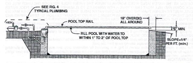
FIG. 2 - PREPARATION FOR INSTALLATION WITHOUT DECKING
