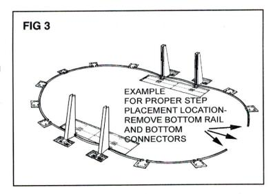
With help, position the step assembly in place and insert the bottom rails onto the bottom rail locators on each side of the step.
