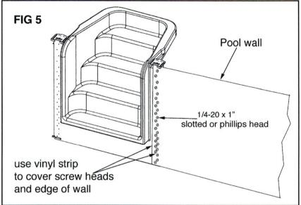
WHEN INSTALLING THE BEAD RECEIVER FOR A BEADED LINER START/STOP THE RECEIVER ON THE OUTSIDE EDGE OF THE STEP AND OVER THE GASKET. YOU WILL NEED TO CUT APPROX 1-1/2" OFF THE TOP OF THE STEP FACEPLATE SO IT WILL FIT AT THE BOTTOM EDGE OF THE BEAD RECEIVER. SEE ILLUSTRATION TO RIGHT.
